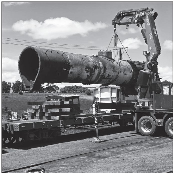
JA1250 boiler and firebox being removed
