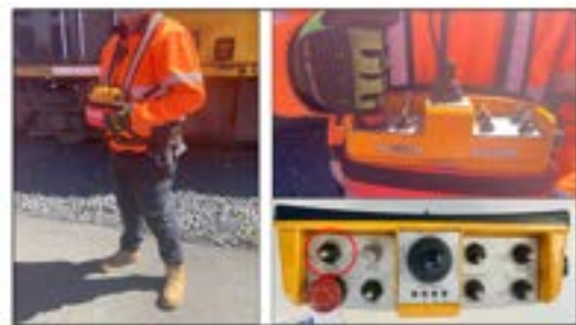
Figure 4. Remote-control pack as worn by an RCO
