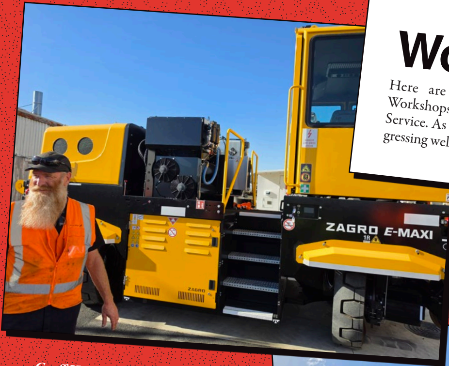
Geoff Ham, Team Leader at Hutt Workshops, shows us a new ESM – Heavy Electric Shunt Vehicle
